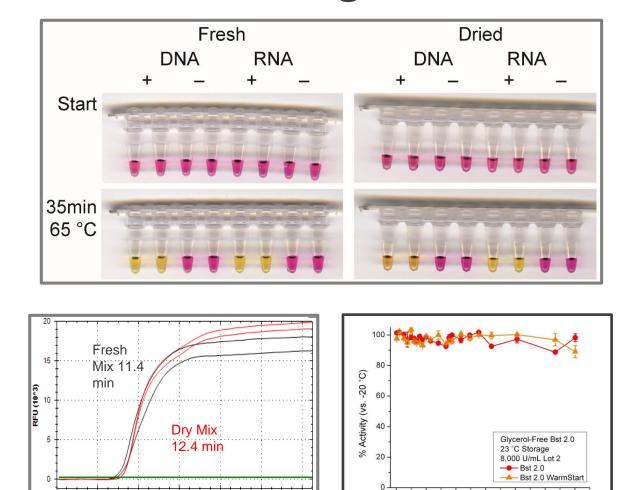
Isothermal and LAMP polymerases (Bst 2.0, Bst 3.0, WarmStart RTx) are stable and available in glycerol-free format. Both LAMP Master Mix formulations can be prepared glycerol-free and are compatible with lyophilization.
