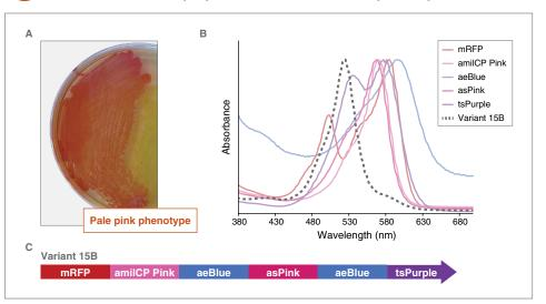
A) Variant 15B shows a pale pink phenotype. B) Variant 15B (dashes) shows a different absorbance profile relative to the parental chromoproteins that make up its parts. The absorbance maximum is shifted and shoulders are absent. C) Sequencing confirms that variant 15B is a chimeric protein comprised of 6 shuffled parts from 5 different proteins.
